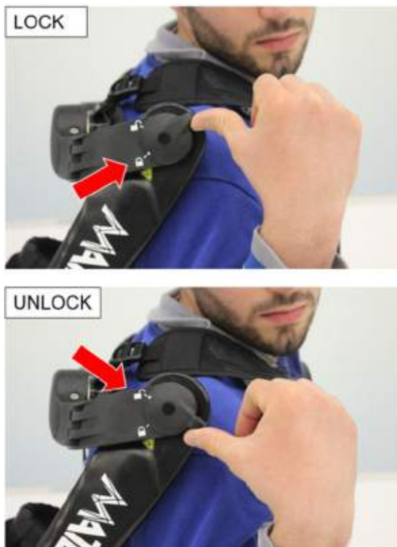
Fig. 3.6 - Torque Generator Box (TGB): locking mechanism
