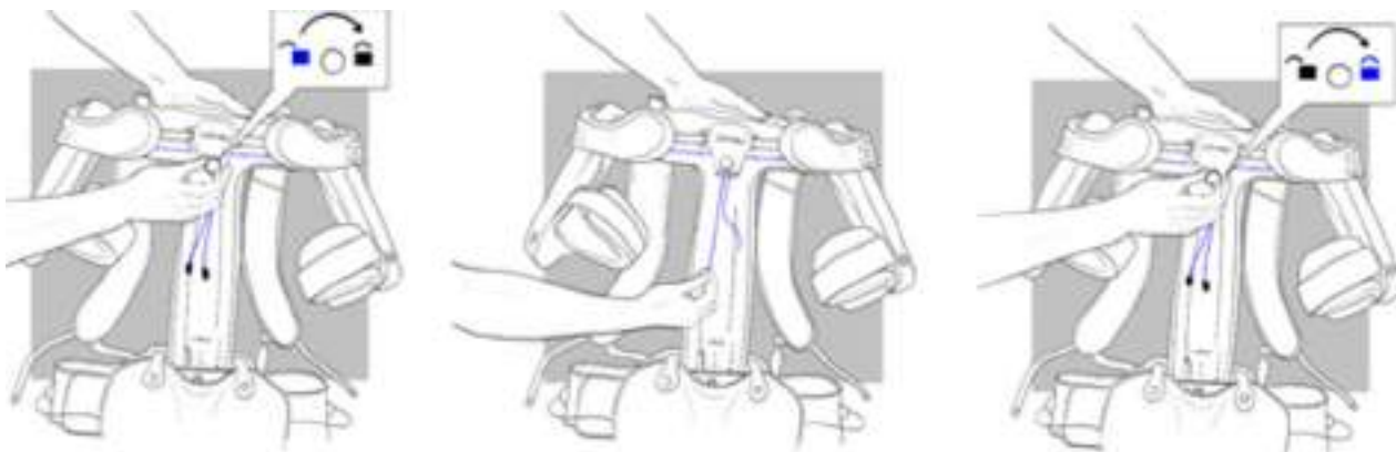
Fig. 4.2 - Rear elastic straps adjustment modes
