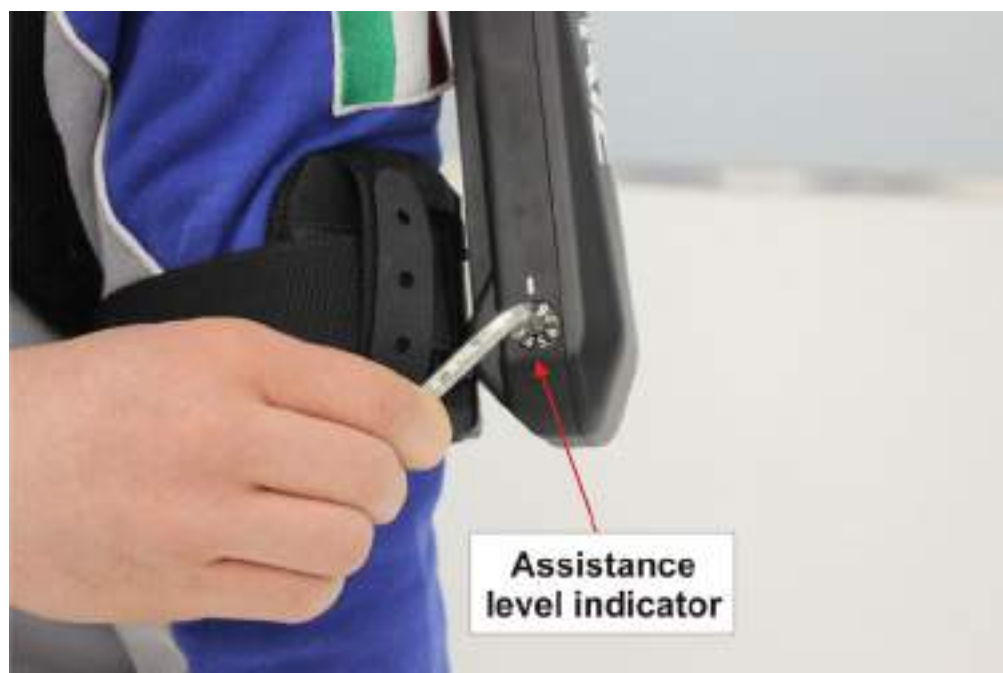
Fig. 4.3 - Close view of the adjustment seat on the Torque Generator Box and the assistance level indicator
