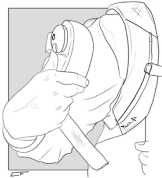
Fig. 5.14 - Locking the TGB locking mechanism
