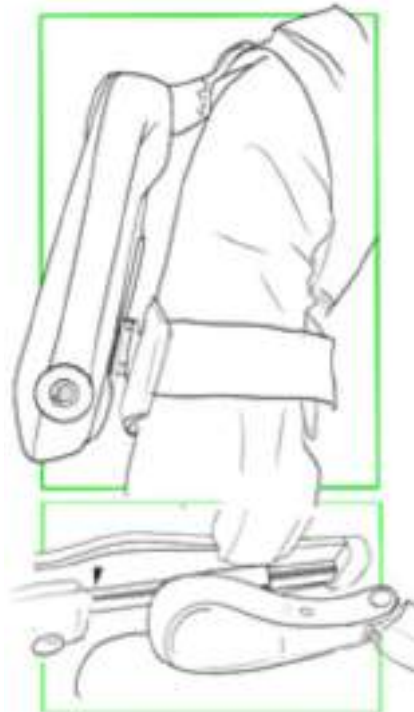
Fig. 6.1 - Detail on the sliding elements of the TGB and the pDOFs
