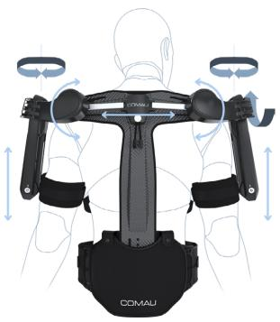
Thanks to a chain of passive degrees of freedom, the flexion-extension rotation axis of the human shoulder is aligned with that of MATE-XT
